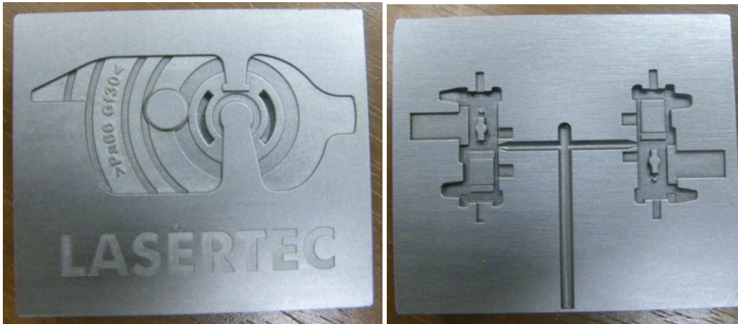
Tool steel Micro-molds fabricated using laser micro milling
